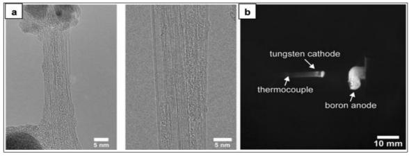
(a) Single and double-walled BNNT synthesised by arc discharge method; and (b) IR image of the cathode and anode electrodes in the chamber. Source: Y.-W. Yeh et al., Stable synthesis of few-layered boron nitride nanotubes by anodic arc discharge. Sci. Rep. 7(1), 3075 (2017)
