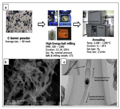
(a) Experimental procedure of ball-milling method. (b) SEM and (c) TEM image of BNNTs produced by the ball-milling method. Cylindrical- and bamboo-like shape of BNNTs is shown in TEM image. Source: J. Kim et al., Synthesis and growth of boron nitride nanotubes by a ball milling—annealing process. Acta Mater. 59(7):2813 (2011)
