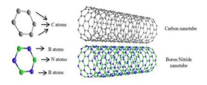
Structure of BNNTs vs CNTs. Source: Comparison of small scale effect theories for buckling analysis of nanobeams, Kadir Mercan & Omer Civalek
